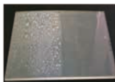
Hydrophilized polypropylene (GGP Treated: Only right-half)
