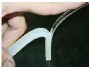
Adhesion between silicone rubber and PP
