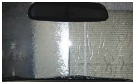
Driving without stress even in heavy rain or at night. (left side is no-coat , right side is coated.)
