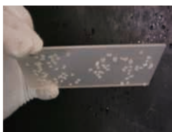
Before GGP-Treated : Polypropylene (adhesion of paper dust by static electricity)
