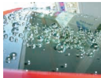
High water-repellent of the contact angle of 110 degrees
