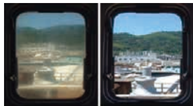
High weather resistant - Possible to use ship. (left side is no-coat , right side is coated.)
