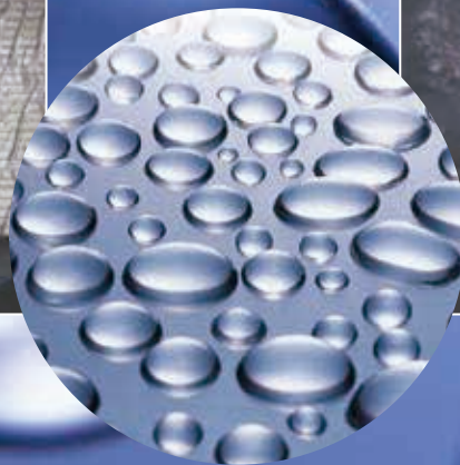
Water-repellent coating on the mirror surface
